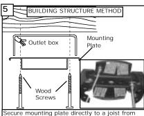
the buliding structure via the two knock out holes on the outlet box. Use only the appropriate wood screws and washers included with your fan. Caution: Wood screws must go through into the building joist.
